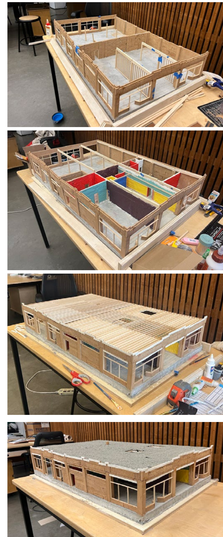
Figure 4.29 Modeling process: wood and brick assembly, plaster and paint, rafter and roof construction
