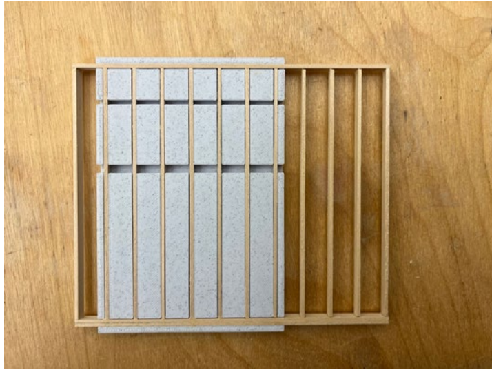
Wall construction made easier with 3D-printed template sized to wall types.
