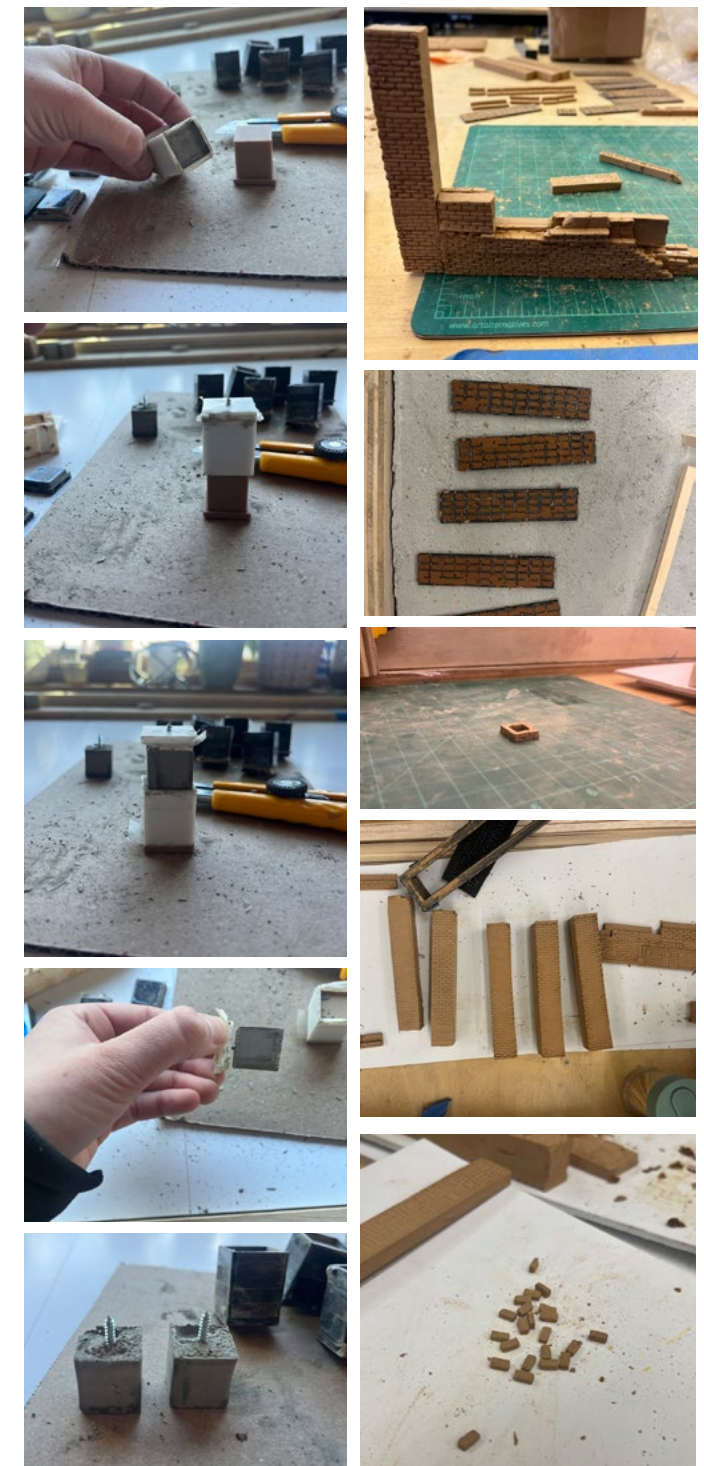
Figure 6.1 Modeling photos: process of casting concrete footers and molding/assembling clay
