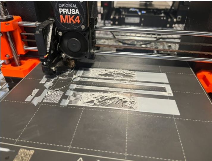
3D printing brick molds.
