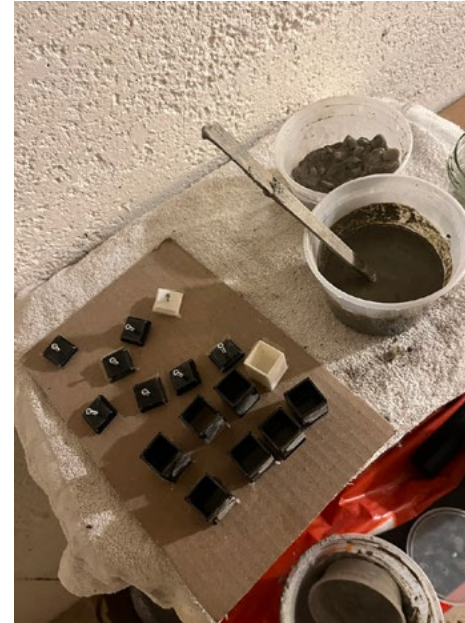
Concrete footers set with screw in 3D-printed molds; wood columns screw into footers.
