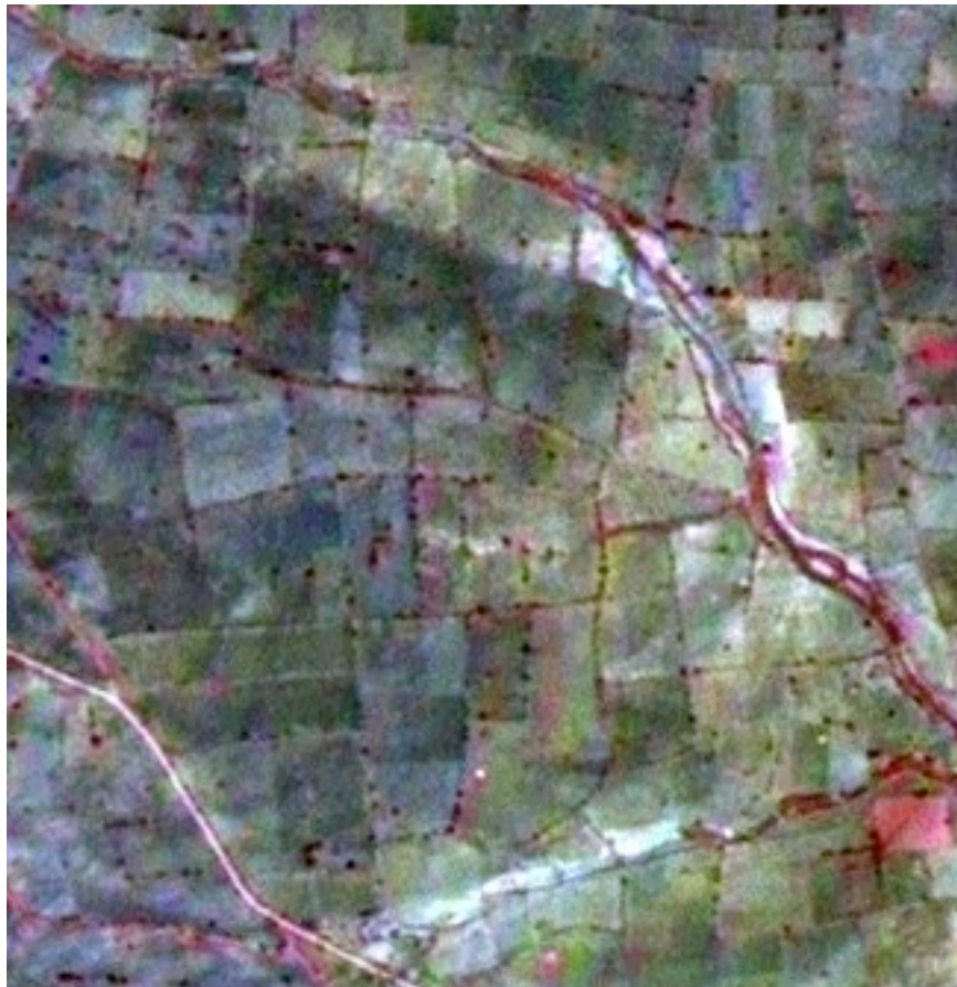
Now we can 'see': 23.5m multi-spectral image merged with 5.8m panchromatic image
