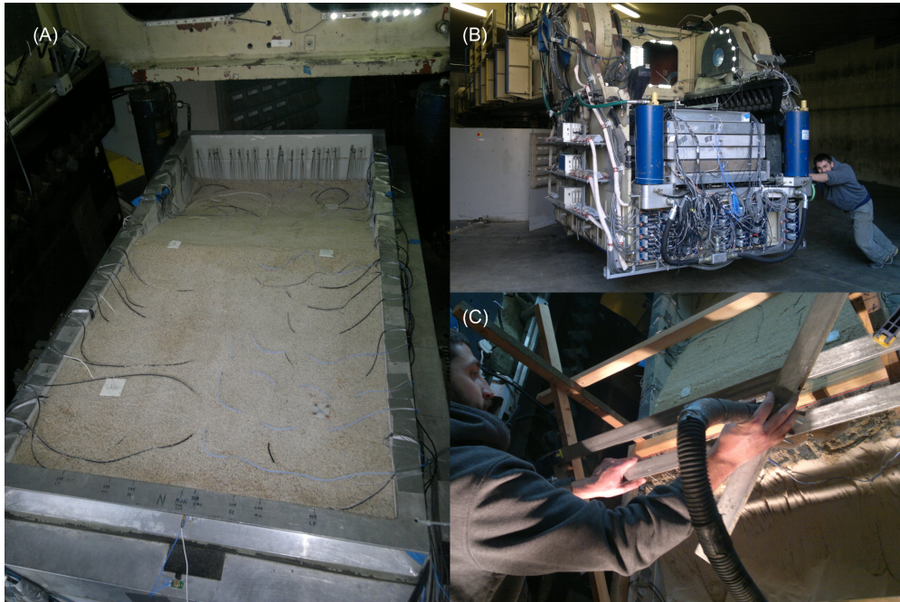
Figure 3.2: (A) The 20 degree slope from above inside the model container. (B) The author pushing the centrifuge bucket attached to the centrifuge arm above. The model container is in between the blue cylindrical compression chambers. (C) The author carving a second slope for the dam-like configuration using a vacuum and guide.
