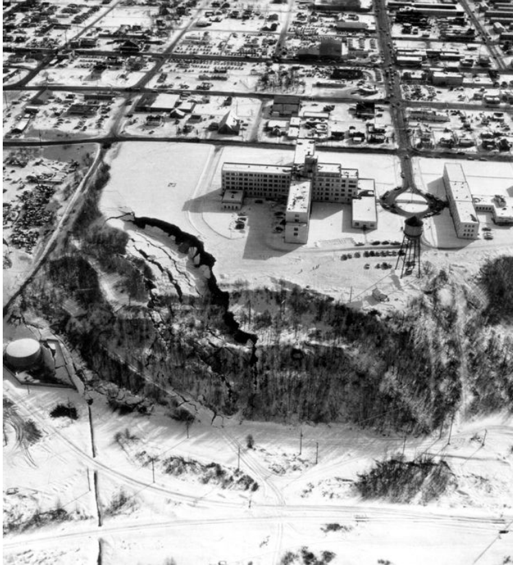
Figure 2.1: Aerial view of the Native Hospital Slide in Anchorage, Alaska, after the 1964 Great Alaskan Earthquake (U.S. Geologic Survey)
