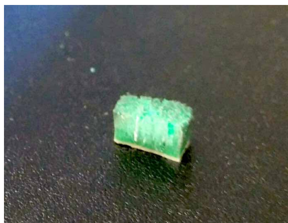
Figure 4.26: Image of normally black LSM-YSZ freeze-cast after sintering under a reducing atmosphere to 1500 °C.
