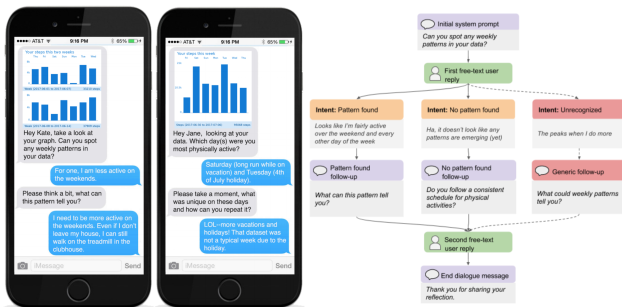
Figure 4.2: Example of an actual user exchanges with our system’s mini-dialogues on the left. On the right a block diagram of an example dynamic mini dialogue with: actual user replies, user intents recognized based on free-text replies, and the system tailored follow-ups. The red boxes represent a path where user reply was not recognized and has been handled by a “generic” (non-tailored) follow-up.
