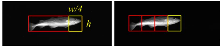
Figure 3.6: Object-height blocks (yellow) on the stereo-rectified left and right image. There are 4 candidates from each of the right target's upright bounding box for the minimum-SAD scheme.
