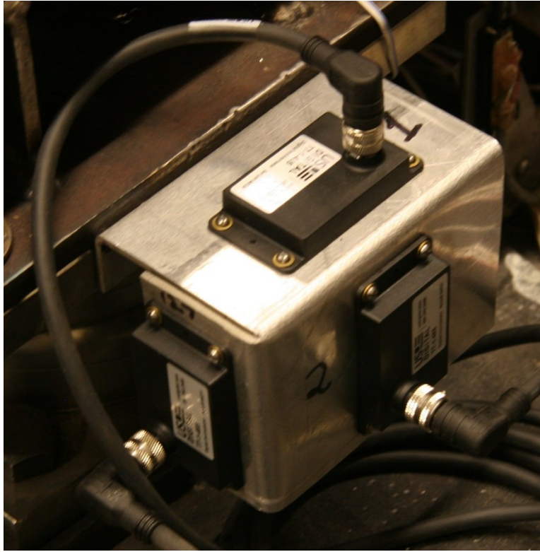
Figure 2-23: Photograph of inclinometer system used to measure bearing rotation.
