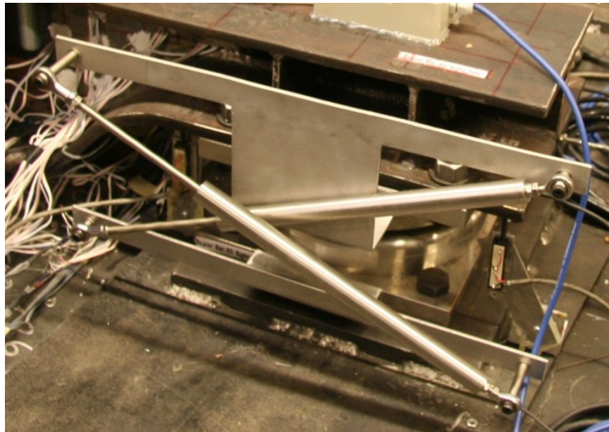
Figure 6-12: Photograph of “crossing” LVDT arrangement
