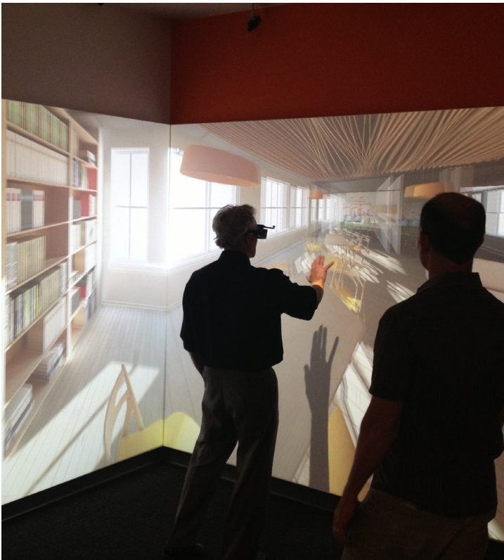
figure.8: CAVE virtual reality being used to view an architectural space
