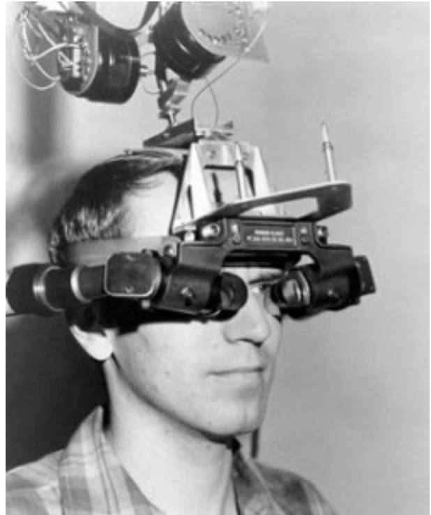
figure.3: Ivan Sutherland's head mounted display.
