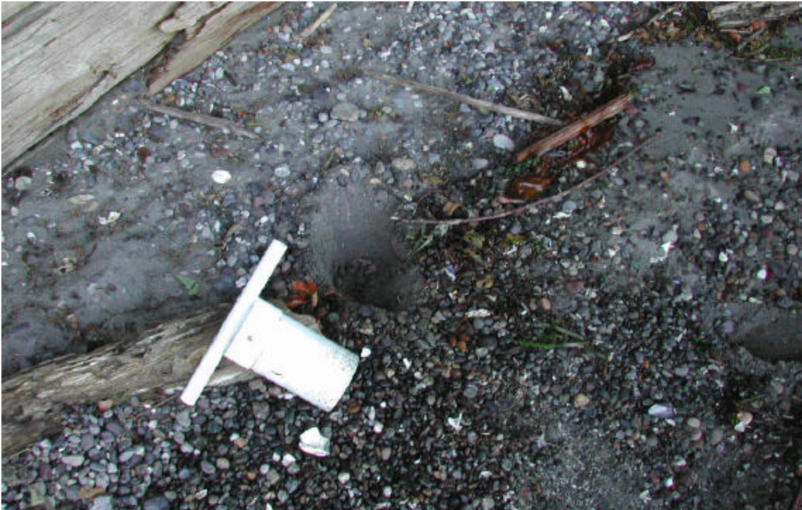
Figure 5. 10 cm diameter core used for sampling benthic invertebrates to a 15 cm depth.
