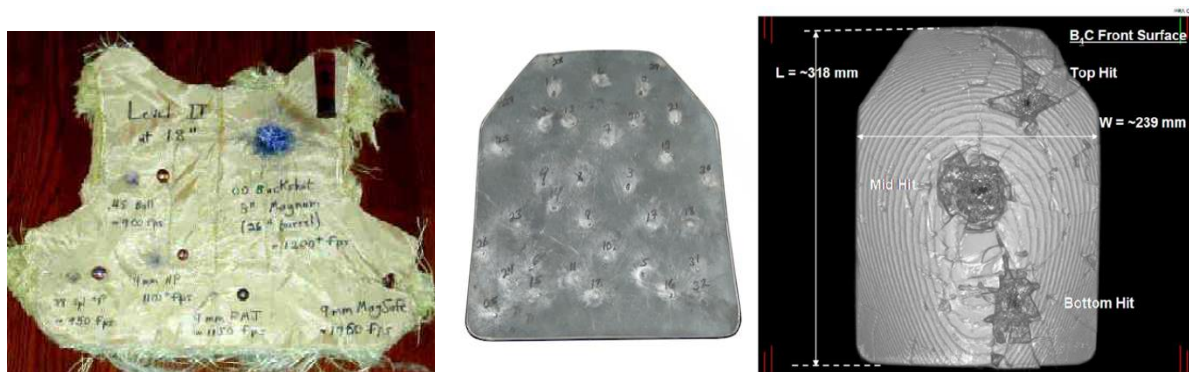
Figure 1.1. Examples of ballistic protection materials post-impact. Left: woven polyaramid fiber vest after impact by multiple small caliber (pistol) bullets. Middle: high strength steel plate that withstood many more impacts. Right: CT image of a boron carbide composite plate with three points of impact [Wells, 2008].
