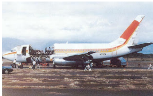
(c) Extended Fuselage Damage of Aloha 243.
