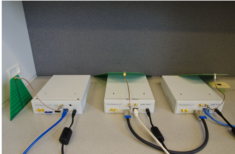
Figure 2.7: Left:PU (USRP2), Middle: Receiver (N210), Right: Transmitter (N210)
