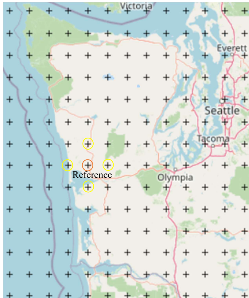
Figure 2.4 Ground Motion Grid B on the Olympic Peninsula with the Reference Point Shown in Orange, and the North, South, East, and West Points shown in Yellow
