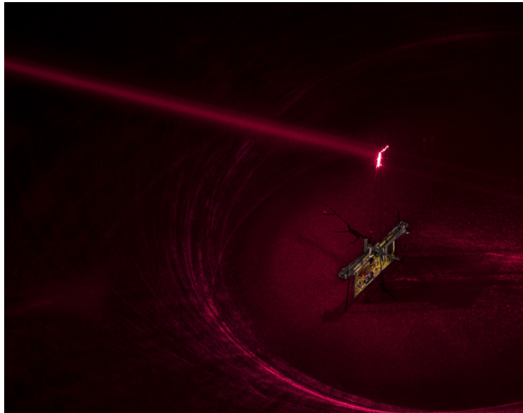
Figure 3.1: Robofly used for [30] equipped with PEU and PV cell, with visible laser showing an example of how the near-infrared beam is aimed at the PV cell for wireless power delivery.
