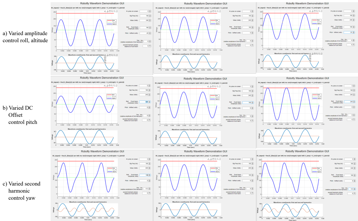
Figure 1.7: Demonstration of the different piezo actuator signals in order to achieve different control actions. [top] 3 cases of varied amplitude, as for roll or altitude control. [center] 3 cases of varied DC offset, as for control of pitch. [bottom] 3 cases of varied second harmonic component, as for yaw control. Variation of the speed of the upstroke relative to the speed of the downstroke causes different drag forces on the wing, creating the yaw moment.
