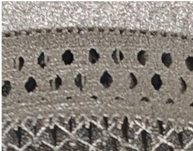
Figure 3.20. As-built support structure manufactured during SARP build.
