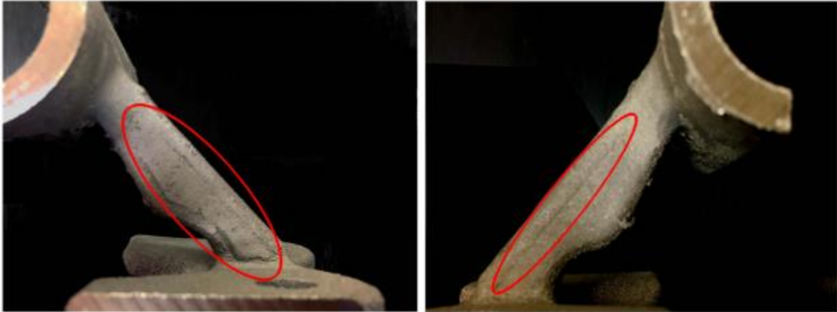
Figure 2.23. Region of a completed part that had undergone swelling [9].
