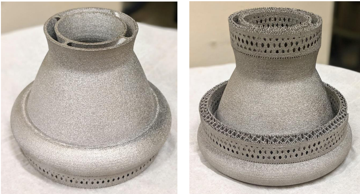
Figure 3.19. Resulting lower nozzle (left) and upper nozzle (right) parts with supports.
