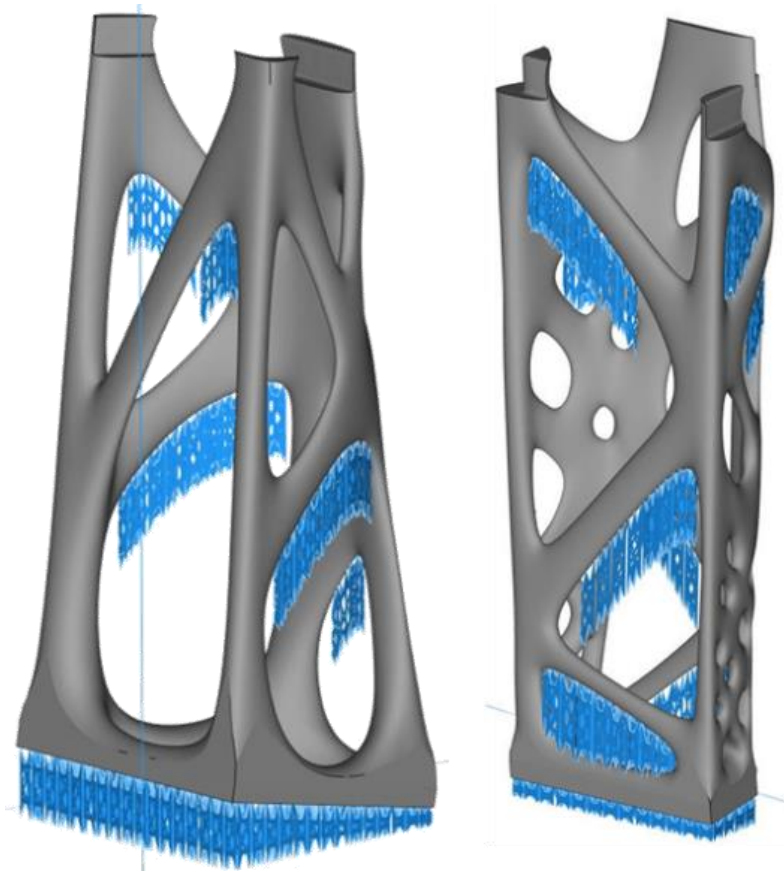
Figure 6.14. Support strategy image for aft/forward section (left/right) final build configuration demonstrating floating support features.
