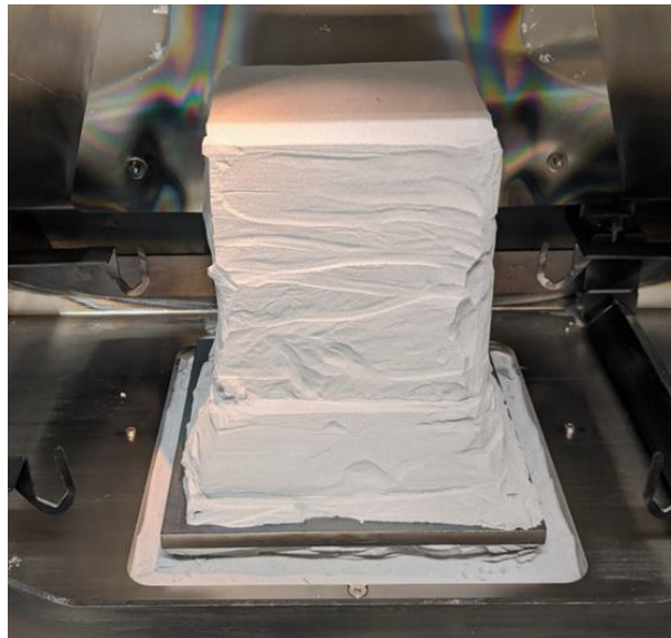
Figure 6.17. The sintered cake of titanium resulting from a build that is ready to be extracted from the Arcam A2X chamber.
