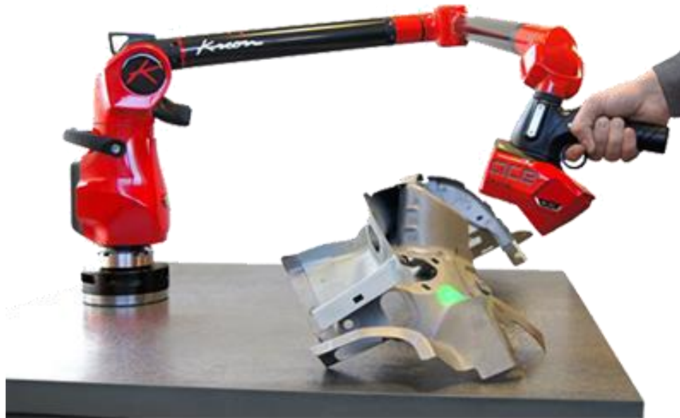
Figure 3.11. Image of a Kreon Ace arm with a Skyline 3D scanner.
