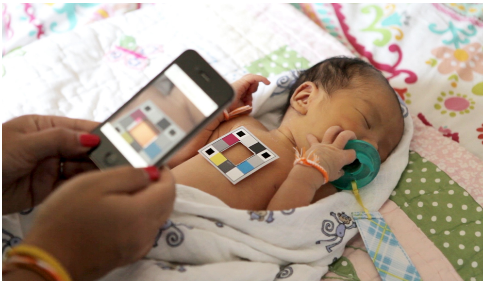
FIGURE 3.2: A photo illustrating how parents or medical practitioners could use BiliCam to monitor a newborn's jaundice with their smartphone.
