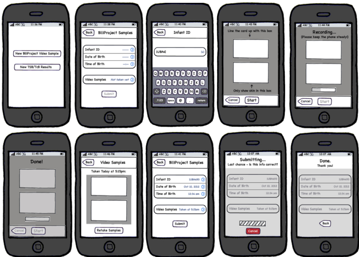
FIGURE 3.5: A subset of paper prototypes from the early design of BiliCam's data collection app.
