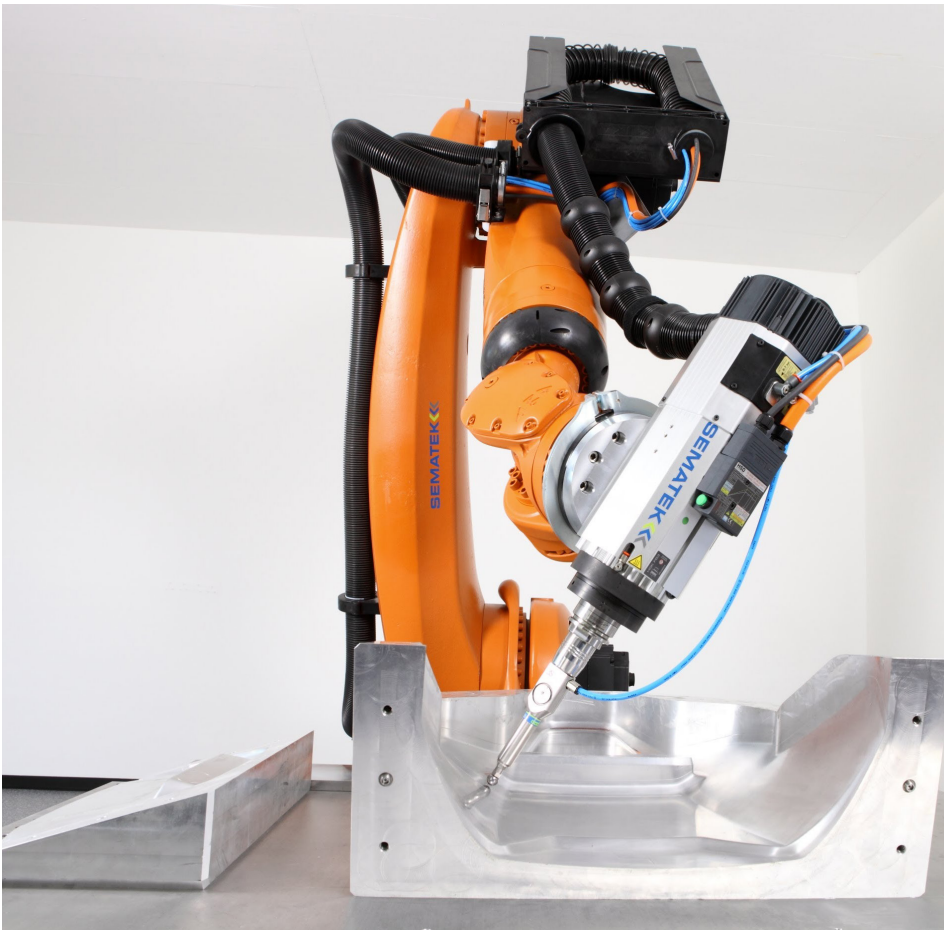
Figure 9: Kuka Robotic Arm milling aluminum.
