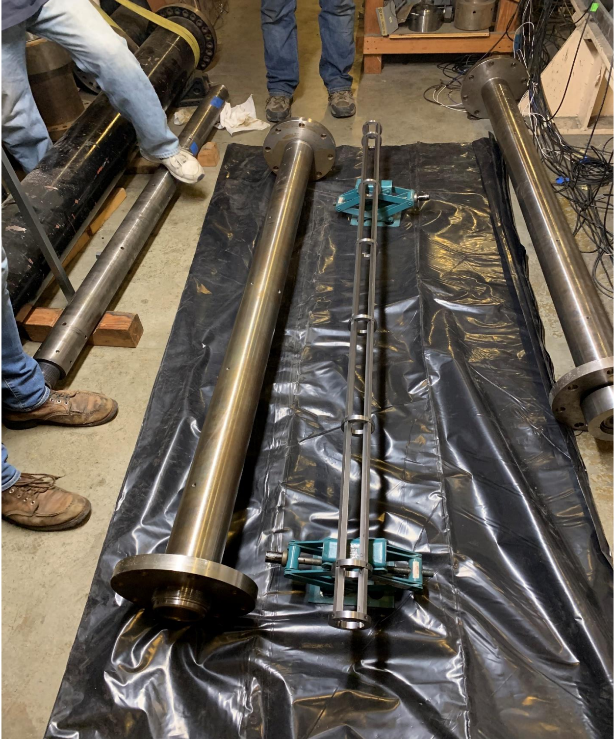
Figure 3. 7: Shell tube with 3" bore and its railed-tube insert
