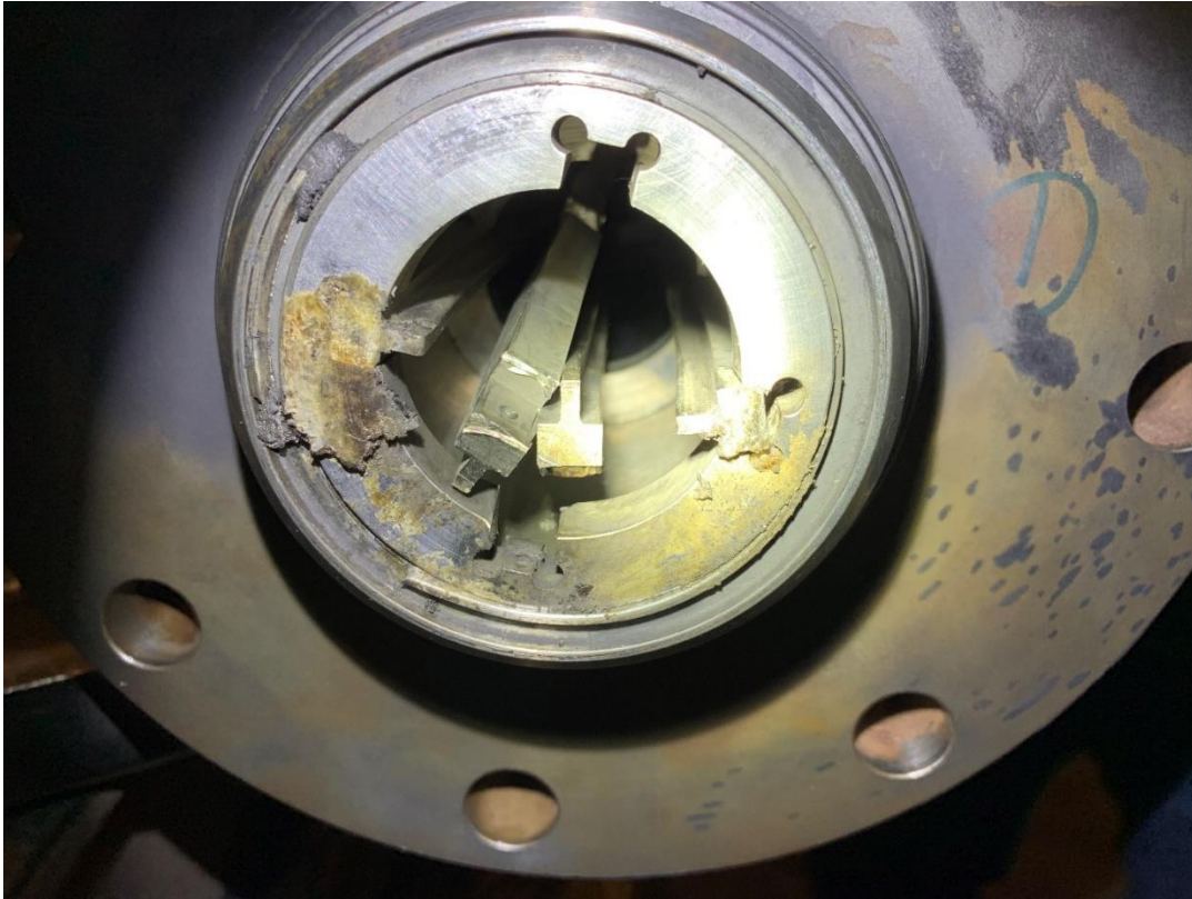
Figure 4. 13: RTRA railed-tube insert and shell tube failure surface
