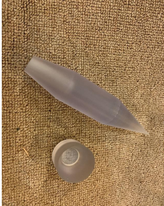
Figure 3. 11: Lexan projectile and piston for the prototype RTRA
