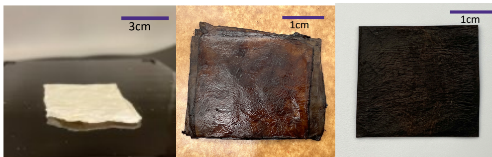
Figure 30. (left) Air dried 4-layer pure BC. (middle) Wet 4-layer BC/lignin. (right) hot-pressed 4-layer BC/lignin with 120C, 5Mpa, 10min.
