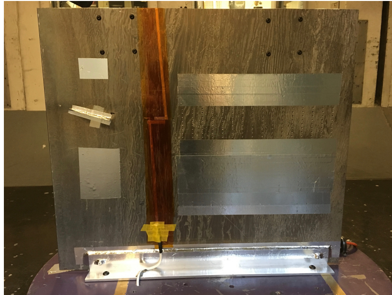
Figure 3.17: The plate with a plasma actuator applied mounted in the wind tunnel.
