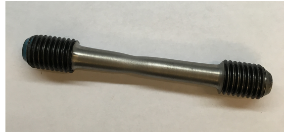
Figure 5.5: Deformed coupon after cyclic tensile axial loading
