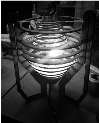
○ Cardboard Prototype with LED Bulb ○ Bulb too Bright & Proportions slightly off
