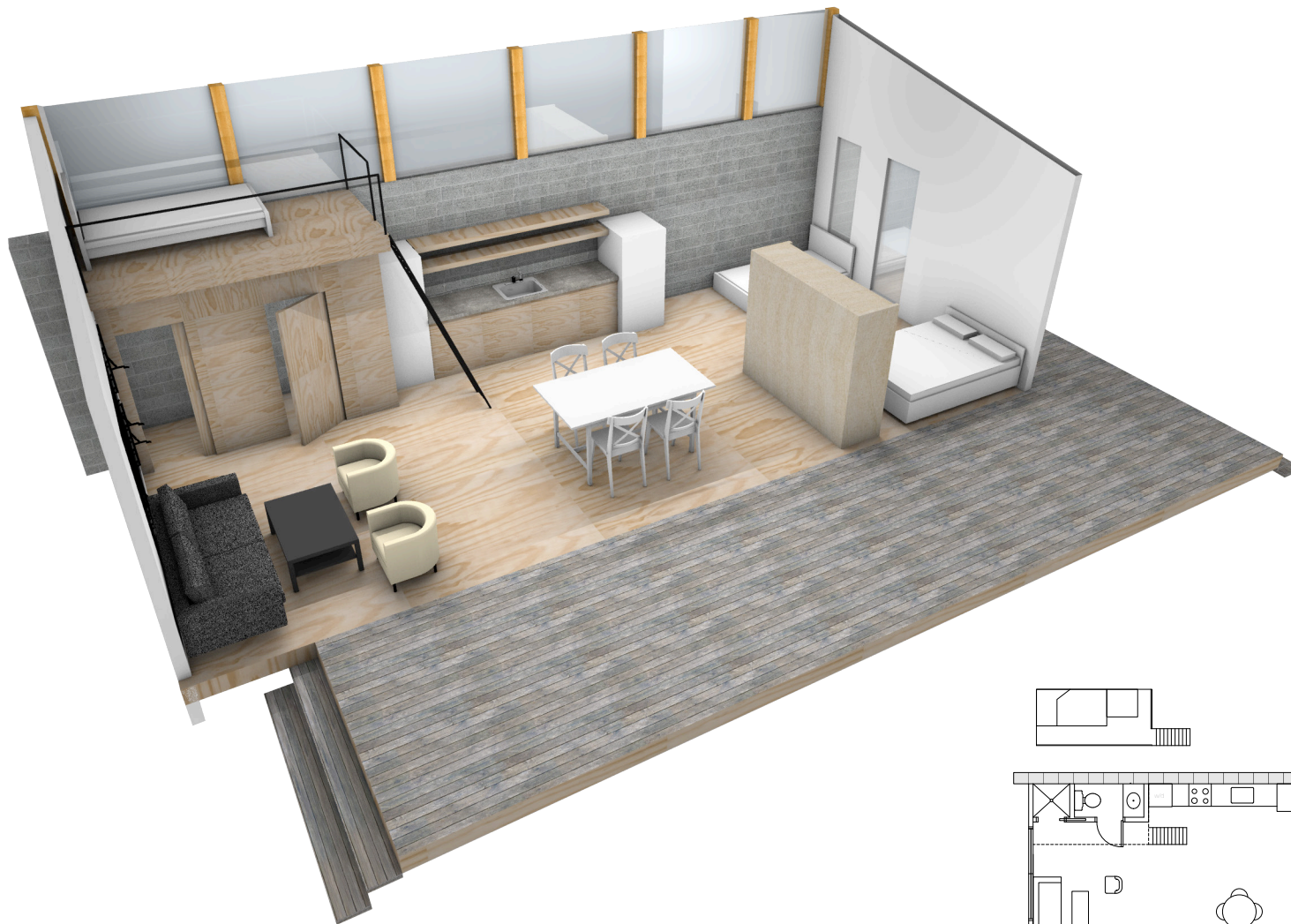
FIGURE 41: PLAN OF SMALL UNIT, THE ONLY TRADITIONAL WALLS ENCLOSE THE BATHROOM AND SHOWER, ALL OTHER PARTITIONS ARE MOVABLE
