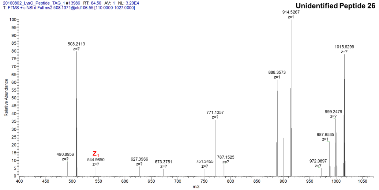
Figure 5.104. ETD-MS2 of LysC-Digested Unidentified Tagged Peptide 26, Undetected by Database but Detected Using In-House Developed Script.
