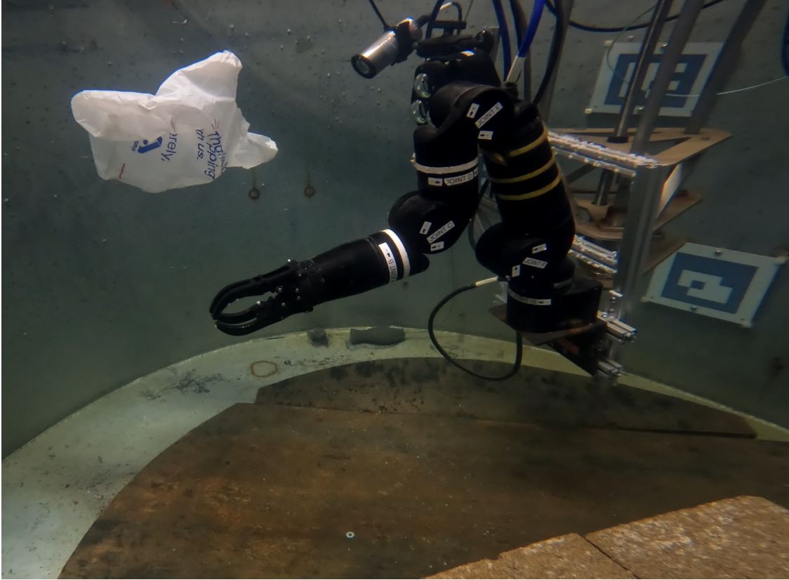
Figure 2.1: Existing underwater manipulation testbed with Bravo Reach 7 arm and stereo camera.
