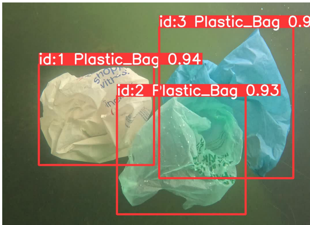
Figure 1.4: Output from DeepSORT tracking showcasing three individual identification tags.
