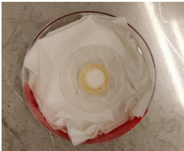
Figure 2.1: The titania membrane with a polymer edge.
