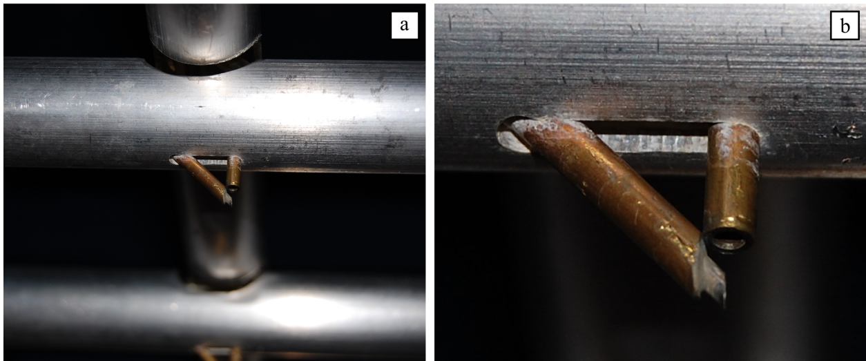
Figure 2.14: Two-fluid atomizers, as installed. Two photos of one of the two-fluid atomizing droplet injectors. (a) One of the grid's eighty-one droplet injectors that are integrated into the intersections of the grid tubes. (b) A close up of the atomizer integrated into the grid.
