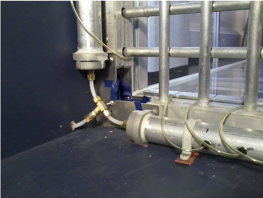
Figure 2.3: Wall jet manifolds. A photo of the manifolds tucked upstream of the grid. The air supply configuration can be seen in the corner.
