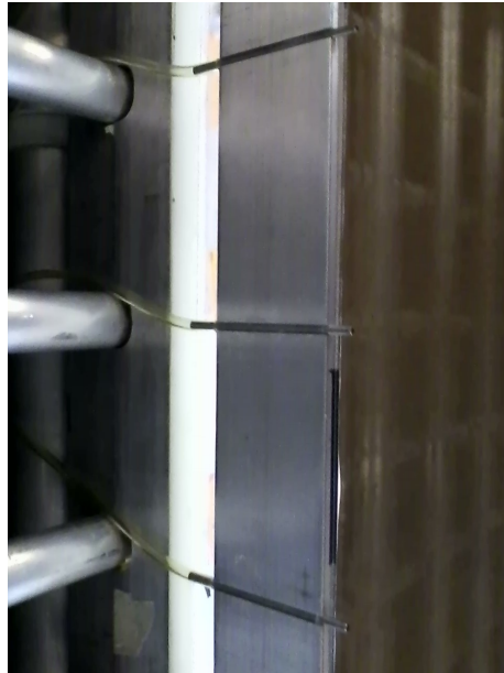
Figure 2.4: Wall jet nozzles. A photo of the wall jet nozzles in the aluminum bar used to hold them on the tunnel wall.
