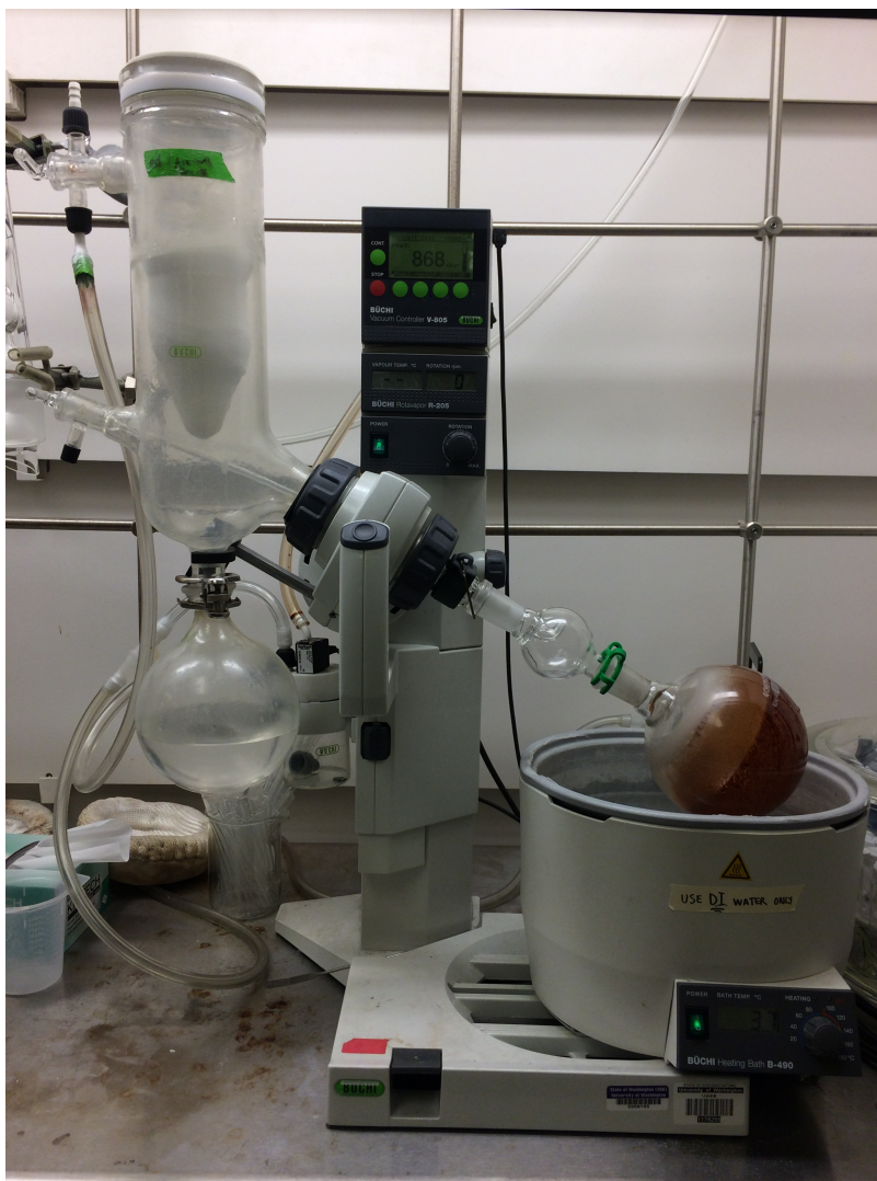
Figure 6. Apparatus for synthesis of trifluoromethyl-functionalized lactide monomer: (concentration of monomer).
