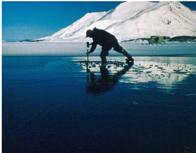
Figure 13. Wilbur Church deploying thermocouples used to measure gravel temperatures in sockeye salmon beach spawning areas.
