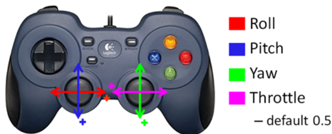
Figure 4.4: Pilot Input via Logitech F310 Gamepad
