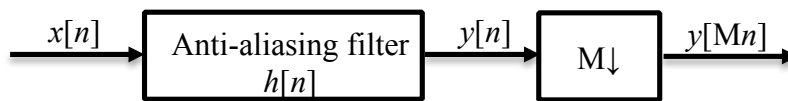
Figure 3.17. Block diagram of a traditional decimation. It involves an anti-aliasing filter and a sample rate decimation of M. The output y is M times slower than the input x.
