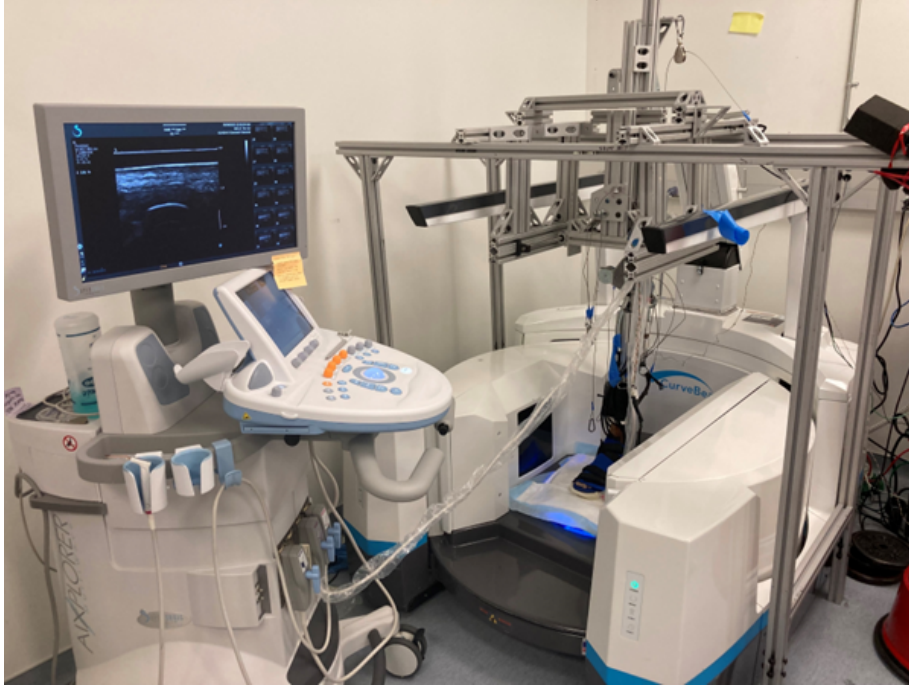
Figure 5: Experimental setup for collecting simultaneous ultrasound using and computed tomography scans inside a LineUp cone-beam, weightbearing CT scanner.
