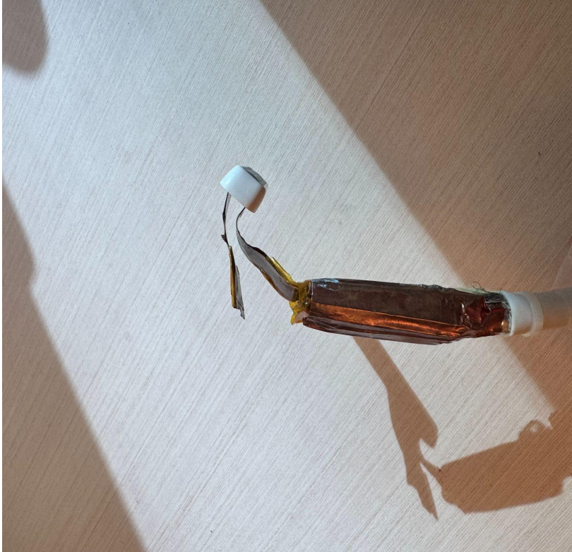
Figure 27: Broken ultrasound probe.
