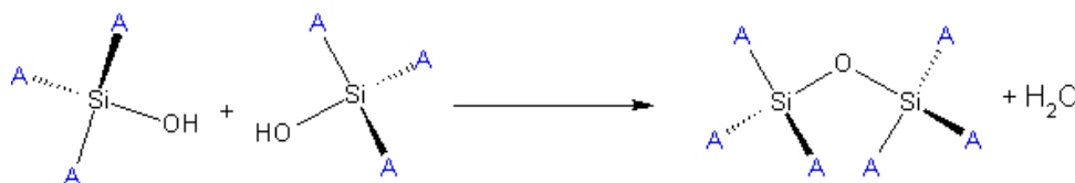
Figure 19: Activation of trimethoxy silanes. “A” represents an arbitrary functional group. The methoxy groups readily leave in the presence of water, leaving highly reactive silanols.
