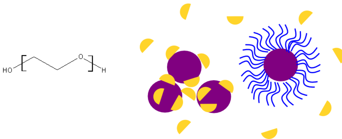
Figure 3: PEG structure (left) and function (right) as a non-fouling agent for nanoparticles. PEG can be chemically conjugated to the surface, incorporated using an amphiphilic version such as PEG stearate, or included pre-fabrication as part of the polymers or lipids that compose the nanoparticle. The hydrophilic PEG localizes to the exterior of the particle and sterically inhibits interactions with the surface, reducing protein deposition and aggregation.
