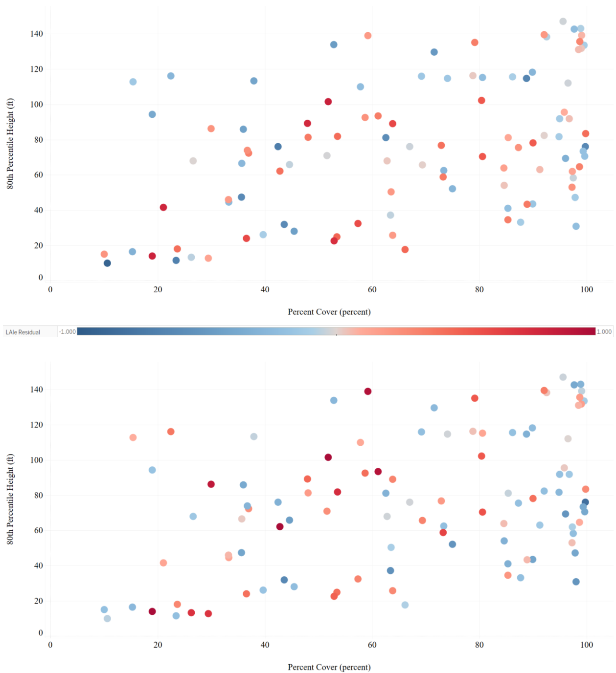
Figure 18. Plotted results of the principal component analysis for measured field plots. Individual observations are colored based on LAI_E Linear Regression estimate residuals for ALS (top) and Sfm (bottom)
