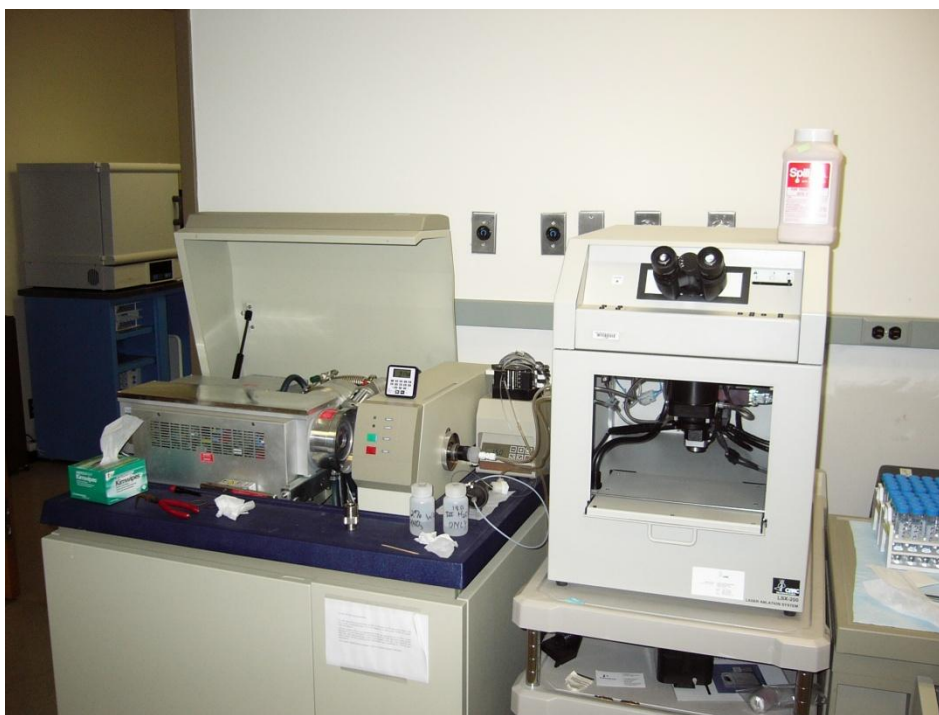
Figure 6.3: LA-ICP-MS system at the Smithsonian Institution Museum Conservation Institute used in this analysis (Photo: S.C. Phillips).
