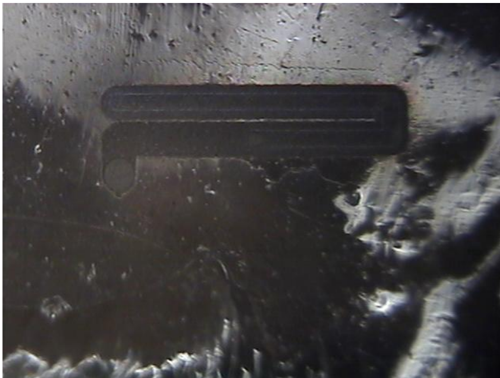
Figure 6.4: Microscope camera screen shot of laser ablation path on an obsidian flake. The ablation channel is approximately 10 microns wide (Photo: S.C. Phillips).
