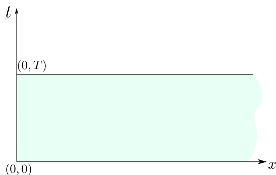
Figure 2.2: The region of integration in the (x, t) plane for boundary-value problems posed on the positive half-line.
