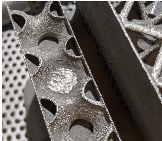
Figure 5.21. Defect discovered on the stress-graded Schwarz Primitive beam specimen.
