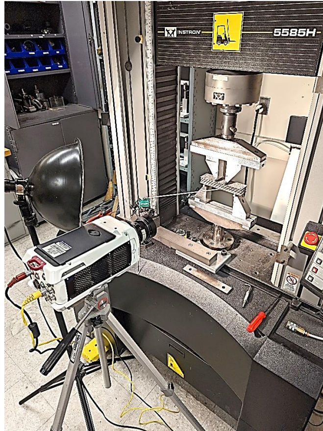
Figure 4.7. Flexure experiment setup showing with the high-speed camera in relation to the load frame.
