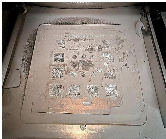
Build 2 Lattice Manufacturing Trial Build 5/1/21 (failure)
