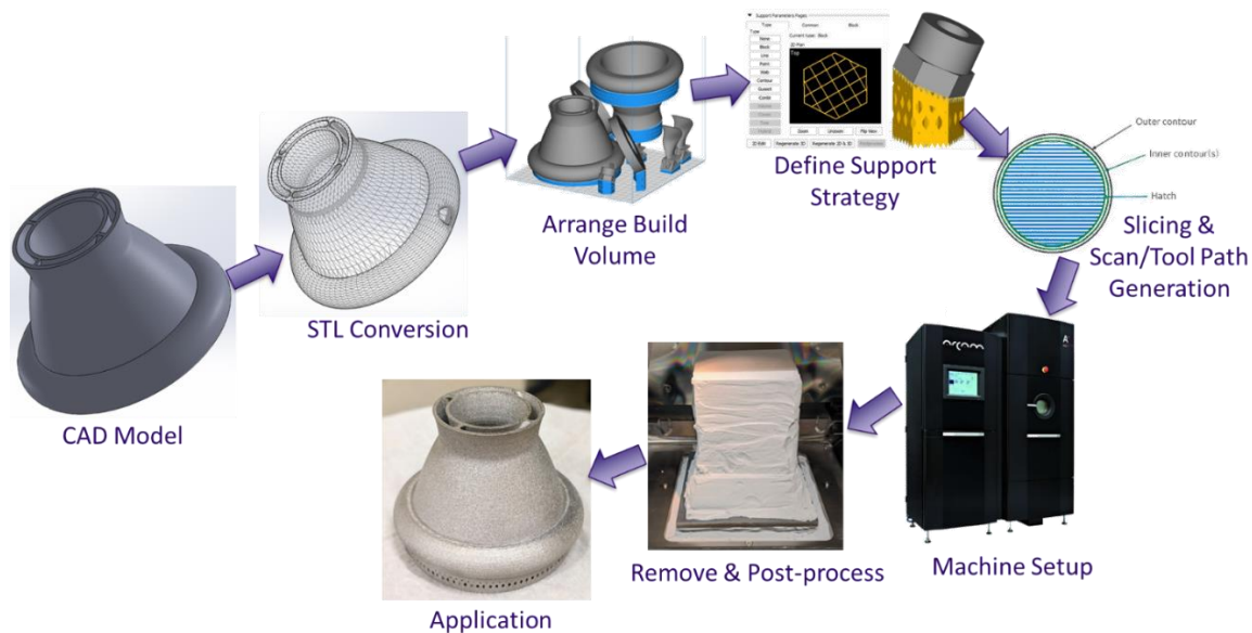
Figure 2.1. EB-PBF process workflow from initial CAD model to fabricated component [34].
