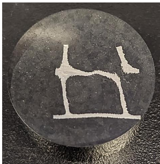
Specimen S1_D (Stress graded Diamond from Build 1) Build Direction Left
