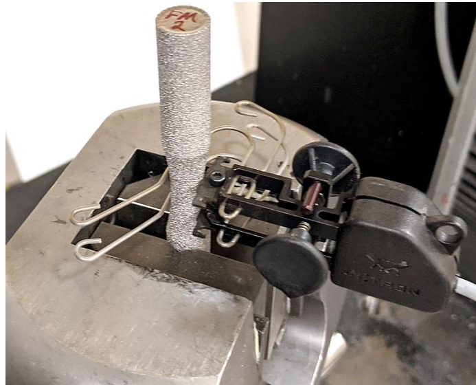
Figure 4.5. ASTM-E466, 9 mm dia. tensile specimen in Instron 5585H loading grip with Instron 2630-101 extensometer attached.
