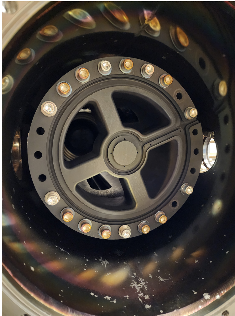
Figure 3.9: The four spoked end wall electrode attached to the outer electrode of ZaP-HD prior to initial testing. This configuration will allow a flow through percentage of 55% while providing an attachment point for the plasma.
