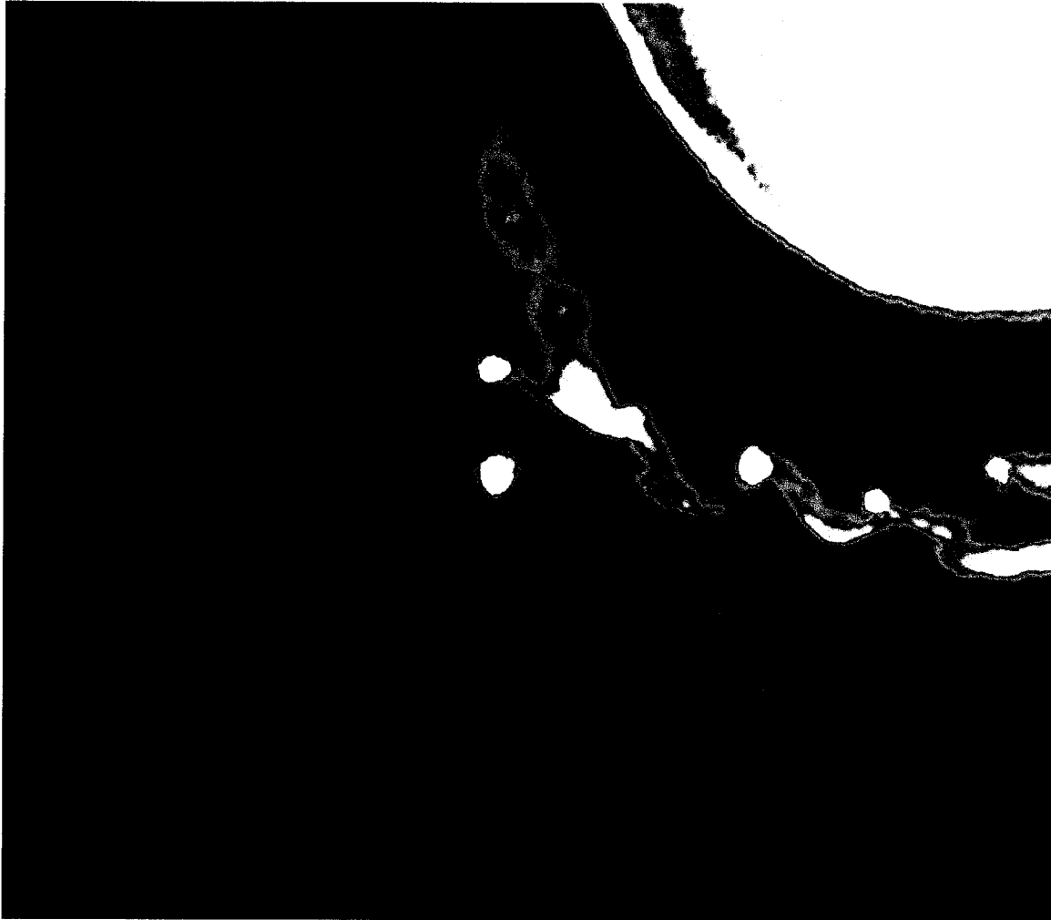
Figure 6.5: A planet formation simulation rendered splatter by SALSA. Each particle can map to multiple pixels, determined by its smoothing length. The value of each pixel is determined by the value of the smoothing kernel at that distance from the center of the particle. Contributions to the same pixel from different particles are combined additively. The pixel value is turned into a color using the WRBB color palette. Compared with Figure 6.3, this picture more closely agrees with how the physical forces are calculated by the simulation tool. It shows the gas to be more like a continuous fluid than the pointlike representation suggests.
