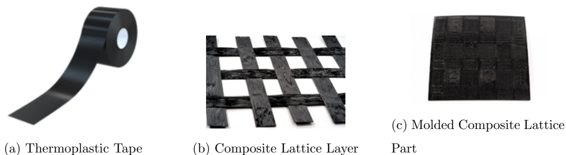
Figure 1.2: Materials and structures used in lattice optimization framework [1]
