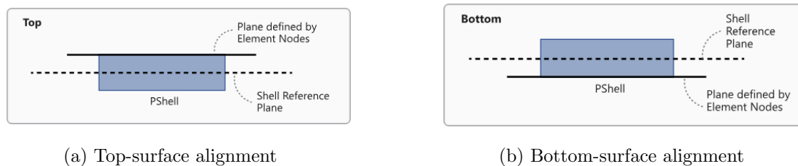
Figure 3.8: Shell element offset options in OptiStruct using the ZOFFS parameter in PSHELL. Left: The top surface of the shell aligns with the node plane, placing the material centroid below the mesh. Right: The bottom surface of the shell aligns with the node plane, placing the centroid above. These offsets are useful when surface-mounted reinforcements (e.g., Weav3D tapes) must be accurately represented in strain response evaluations.
