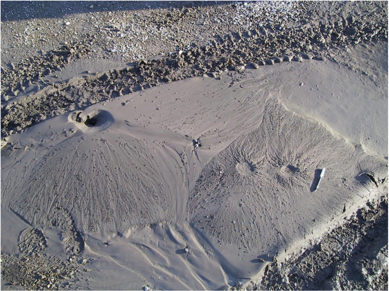
Figure 6- Photo showing multiple sand boils at one location. Pen for scale. Photo provided by Kathy Troost.
