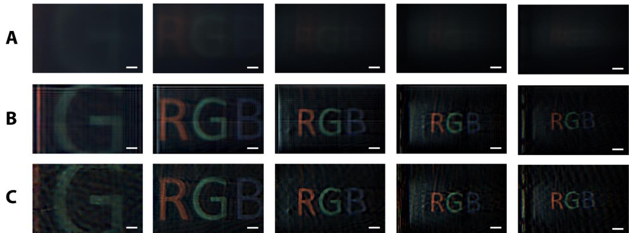
Figure 5.15. Deconvolution Algorithm Comparison. Raw images captured of RGB characters are shown (A) for five different zoom levels and images after post-processing with Wiener deconvolution (B) and using the TV-regularized algorithm of the main text (C) are also shown. Wiener deconvolution in this work offers a 113x average computation time speedup but for high magnification levels, ringing artifacts become more significant.
