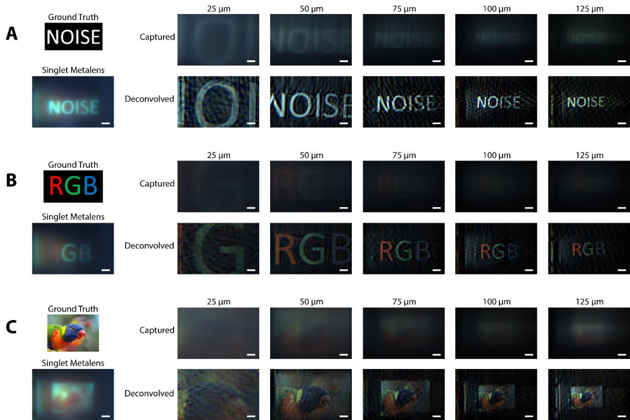
Figure 5.6. White Light Imaging. Images are shown depicting the ground truth objects that were imaged, including “NOISE” text (A), “RGB” text (B), and a colorful bird (C). Also shown are images captured using the 1.5 mm singlet metalens under white light for comparison, and the images from the Alvarez EDOF metalens before and after deconvolution for five different lateral displacements ranging from 25\ \mu\text{m} to 125\ \mu\text{m} from left to right. Scale bar 62\ \mu\text{m} in all images.
