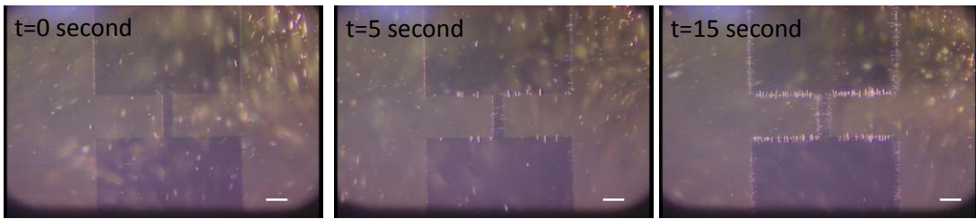
Figure 5. Sequential images of 15 \mu\text{m} -long nanowires deposition on the planar electrode using Dielectrophoresis. Applied voltage is 20 Vpp (peak to peak voltage) at 5 MHz. The scale bar is 100 \mu\text{m} .
