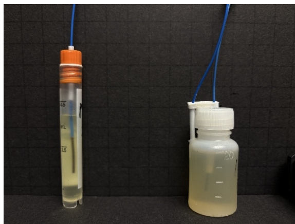
Figure 6-1. 4 mL and 20 mL sample holder and optic fiber temperature sensor setup
