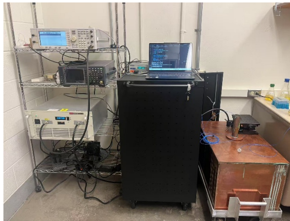
Figure 5-7. 434MHz SMER system with auto-tracking system included. From left to right are the signal generator, amplifier, auto-tracking system, and cavity system.
