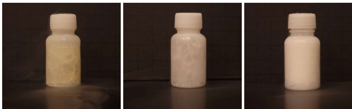
Figure 6-3 Vitrification solution directly Plugged into LN2 tank showing crack. (left)10D37.5PVP (10kDa), (middle) 40D6PVP (360kDa, Sigma), (Right) 40D6PVP (360kDa, Thermofisher).
