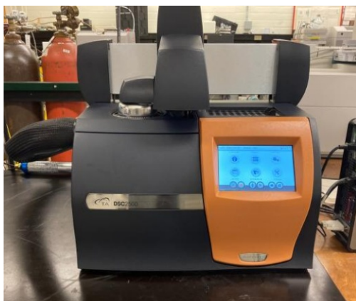
Figure 3-1. DSC equipment and its specification. TA Discovery DSC 2500 with auto loading system for thermal property measurement and its specification
