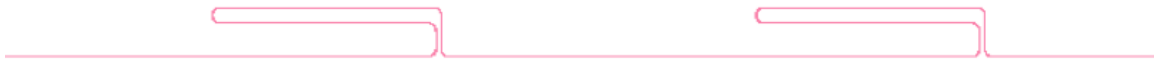
Figure 3.7: Example layout of an optical delay line in the case where the RF and optical propagation speeds are unmatched.
