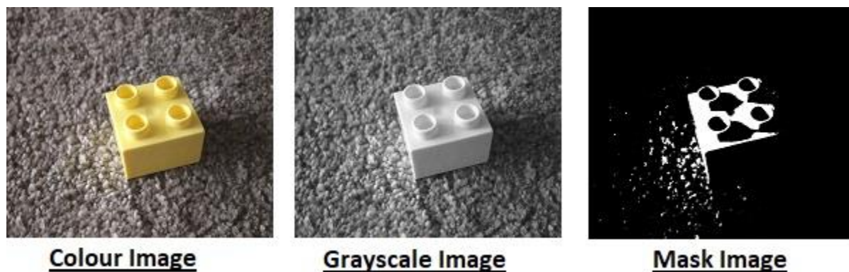
Figure 7: Example of image thresholding.
