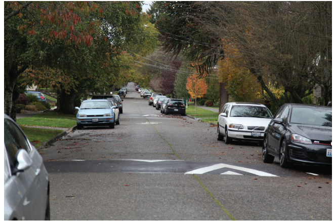
A typical neighborhood greenway street with speed humps and sharrows along the route.
