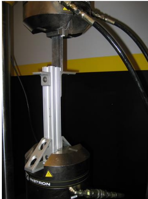
Figure A1.18. Test of sliding force resistance on a 4301 bracket.
