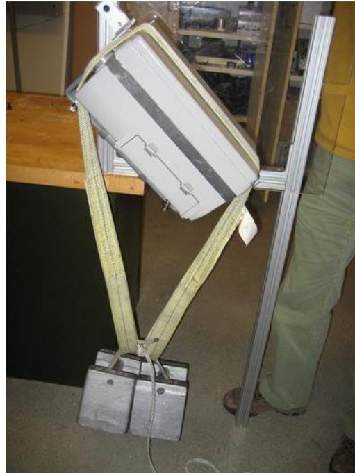
Figure A1.31. Scope mounted with loads equivalent to a 9 g forward acceleration being applied.
