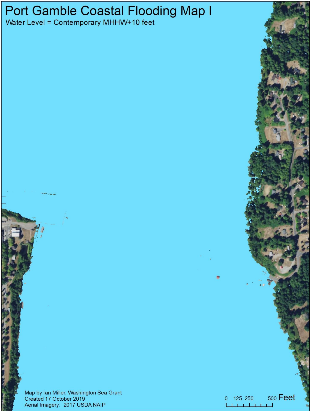
Figure C9. Inundation map showing estimated flooding extent of Point Julia at current MHHW plus 10 feet.
