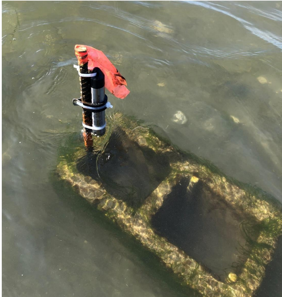
Figure 24. One of the Onset water loggers deployed on the tidal platform of the PGST beaches. I used the water loggers to calculate water levels along PGST beaches to compare to permanent tide gauges at Seattle and Port Townsend.
