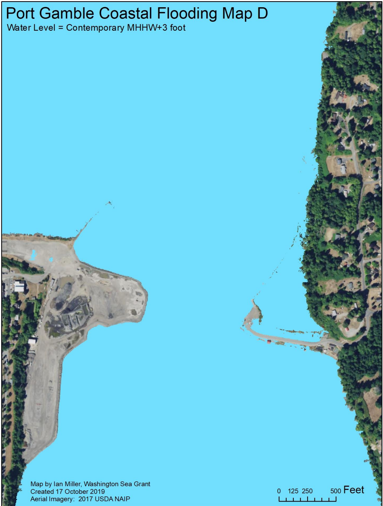
Figure C4. Inundation map showing estimated flooding extent of Point Julia at current MHHW plus 3 feet.
