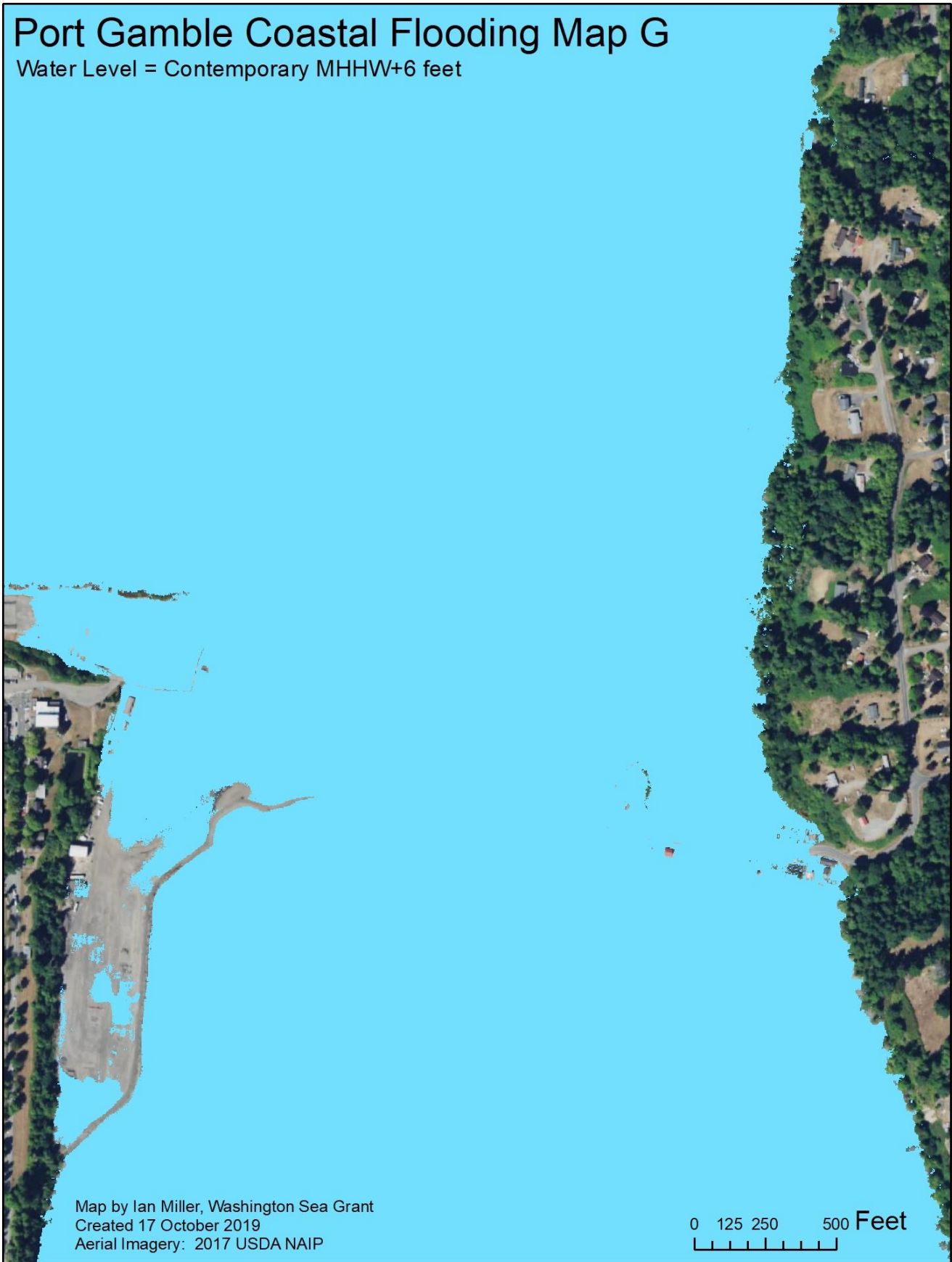
Figure C7. Inundation map showing estimated flooding extent of Point Julia at current MHHW plus 6 feet.
