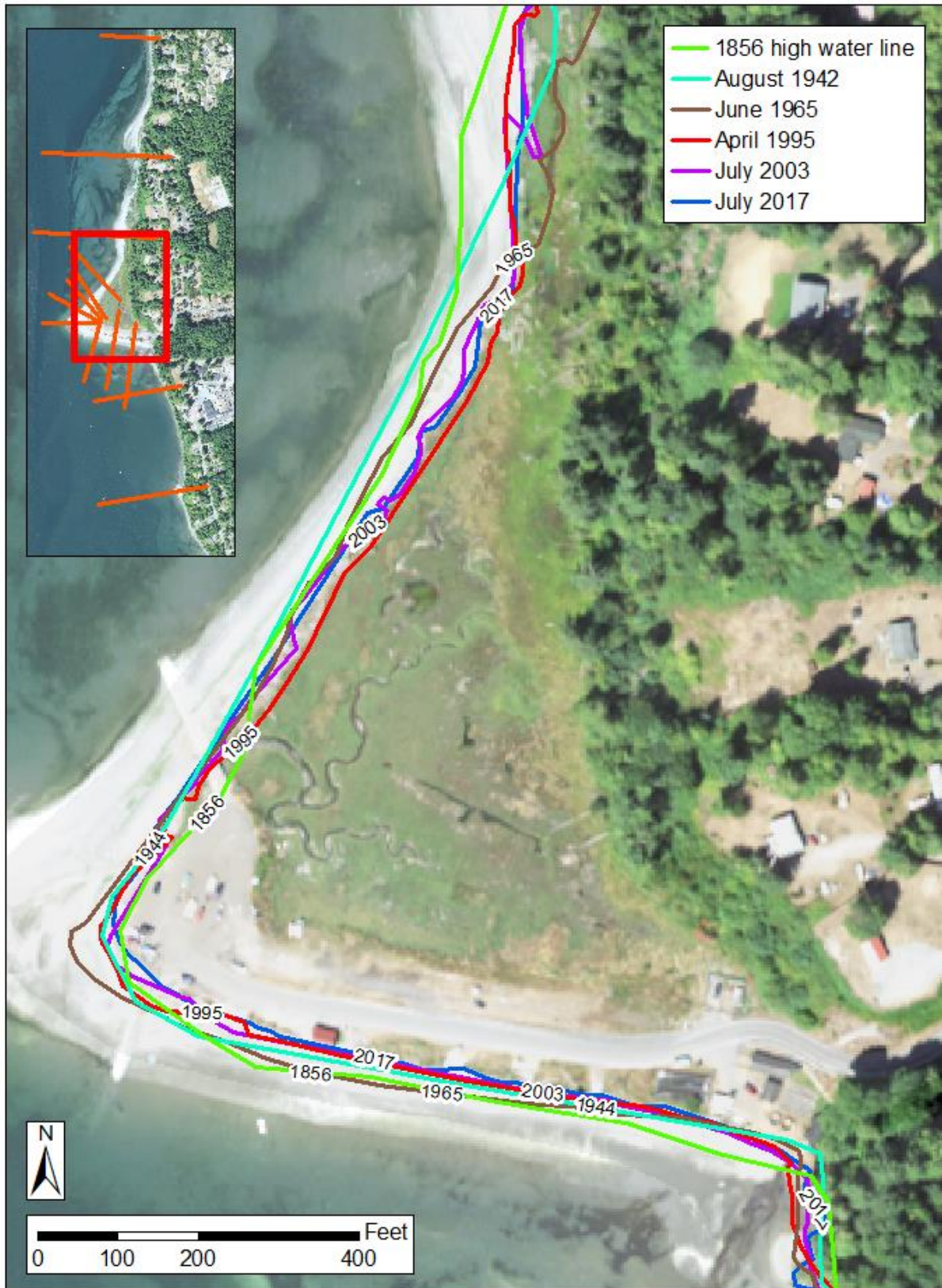
Figure 9. Shoreline change map of Point Julia. These data show a potential pattern of sea level rise with slight landward movement of the shoreline on the south side of Point Julia. I mapped shoreline from 1856 T-sheet high water line and vegetation lines from aerial imagery available at the University of Washington Libraries. Base map aerial imagery from 2017 USDA NAIP.
